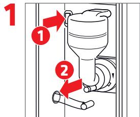
Open front door, switch off, remove tube
