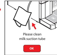
A reminder is displayed to clean the milk delivery tube. Press “OK”
