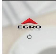
The "POWER ON" screen is shown. Touch the "O" symbol to open the initial screen
