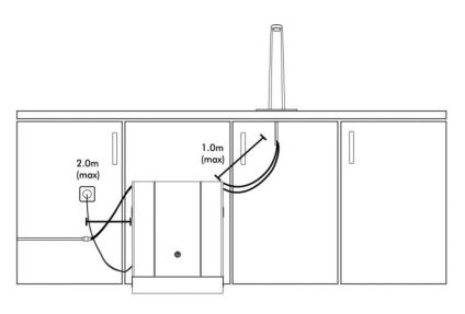
Minimum space for **all equipment** under the counter is a 500 mm kitchen unit, with the full height allowance (no drawer).
