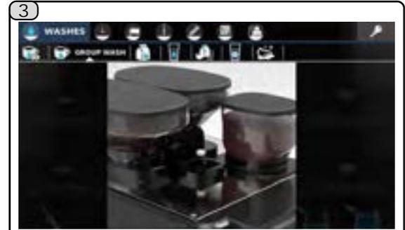
Insert a cleaning tablet into the tube, as shown on the touch screen.
