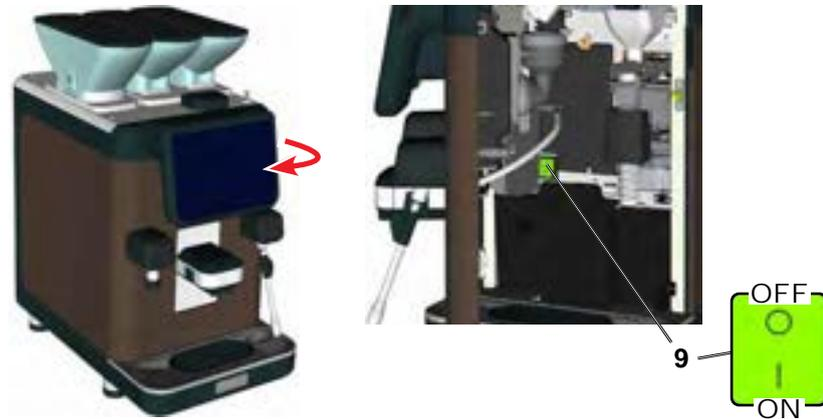
Fully shut down the machine pressing the main switch (9) into **OFF**
