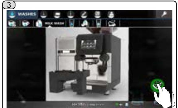
3 The steps for performing a milk wash are shown on the touch screen; at the end of each phase, press the icon
