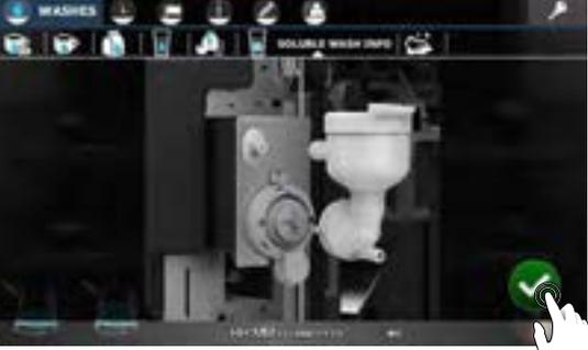
The steps to perform in cleaning the mixer are shown on the touch screen. After each instruction, press the
