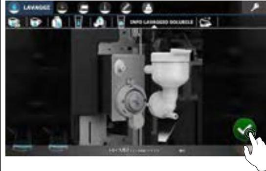
This sequence for cleaning the mixer is shown on the touch screen. After completing each step, press the
