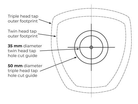
The hole in the worktop required to install the tap will vary based on whether you are installing the **C2 (twin head)** or **C3 (triple head)**.
