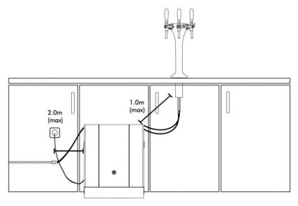
Minimum space for **all equipment** under the counter is a 500 mm kitchen unit, with the full height allowance (no drawer).
