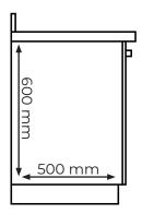
Minimum space for all equipment and a scale management filter under the counter is a 600 mm kitchen unit, with a minimum height of 600 mm.
