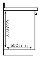
Minimum space for all equipment and a scale management filter under the counter is a 600 mm kitchen unit, with the full height allowance (no drawer).
