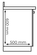
Minimum space for all equipment, CO<sub>2</sub> cannister and a scale management filter under the counter is a 600 mm kitchen unit, with a minimum height of 600 mm.
